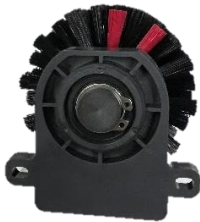
The bristles reach to the red line Excessive wear
